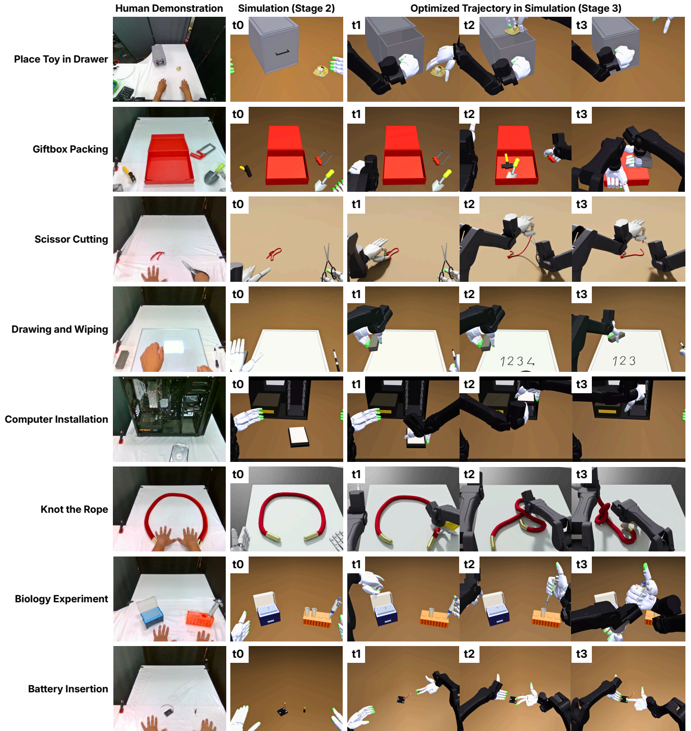
Fig. 7: Additional examples of property-based simulation reconstruction in Stage 2 and robot trajectory optimization in simulation in Stage 3. Column 1 shows the recorded human demonstration, and Column 2 shows the corresponding simulation scene reconstructed in Stage 2. Column 3-5 show representative frames t_0 - t_3 from the robot trajectory optimized in simulation from Stage 3.
